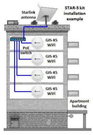
The GIS-K5 wireless Internet controllers connect to the ISP router via the PoE switch included. The GIS-K5 wireless controllers are installed throughout the building to provide good wireless coverage. Additional STAR-5 and STAR-9 kits can be added for very large buildings.
